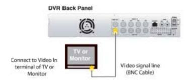
To display the DVR's picture, the video output signal need to be transferred to your TV set or monitor. Any TV set that has a VIDEO INPUT terminal is suitable for displaying the picture. The figure above shows the video signal line connection.
